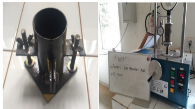
Figure 3. Making a test model with static compaction
